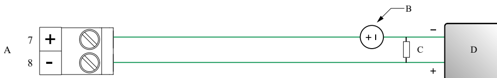
Figure 4-15: Frequency output wiring (externally powered)
