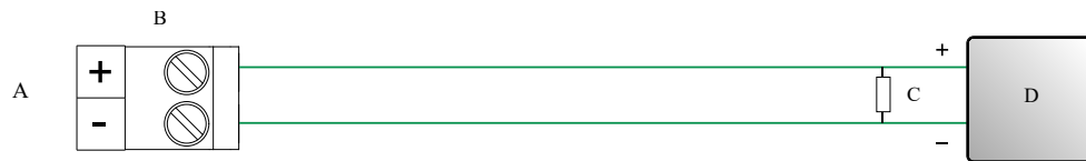
Figure 4-3: mA output wiring (internally powered)
