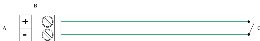
Figure 4-25: Discrete input wiring (internally powered)
