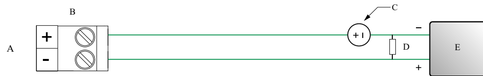
Figure 4-18: Discrete output wiring (externally powered)
