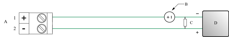
Figure 4-7: mA/HART output wiring (externally powered)
